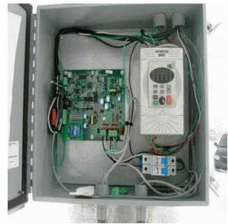
Figure 9 – NEMA Enclosure with Control Electronics
