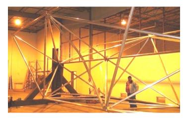
Figure 5 – Space frame load test. Note buckled member in middle of picture.
