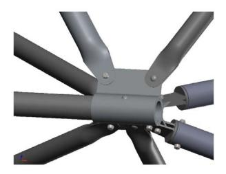
Figure 4 – Solid model of a typical joint on the SkyTrough
