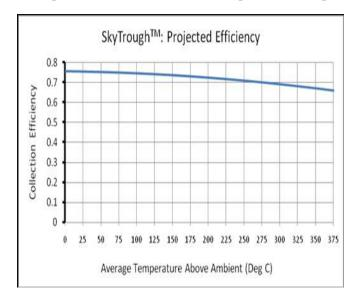
material characterizations, receiver thermal testing, and drive/control testing. Based on these tests, the projected efficiency of the SkyTrough<sup>TM</sup> is shown below in Figure 11, for a direct normal irradiance of 1000 W/m<sup>2</sup>, at normal incidence.
