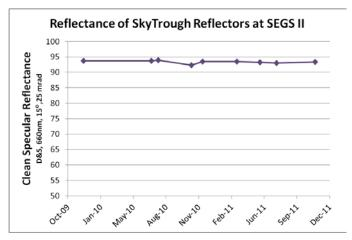
FIGURE 5. Specular reflectance of the SkyTrough at SEGSII.
