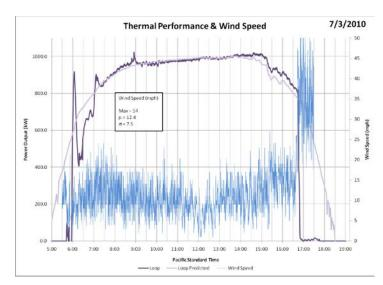
FIGURE 4. Thermal performance, predicted and measured, with wind speed for a single day.
