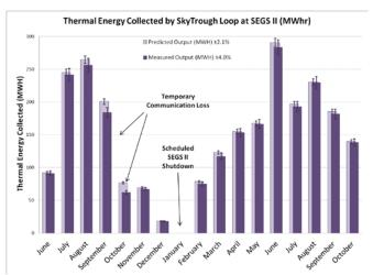
FIGURE 4. Measured compared to predicted performance of SkyTrough loop by month.
