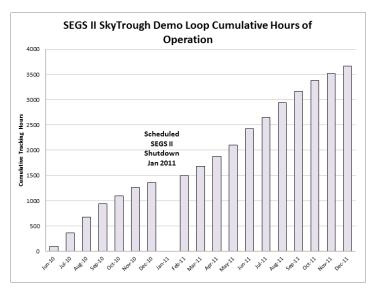
FIGURE 3. SkyTrough cumulative hours of operation, since installation of the data acquisition system.
