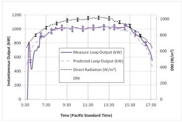
FIGURE 2. Performance of SkyTrough loop over the course of a day, measured and predicted.
