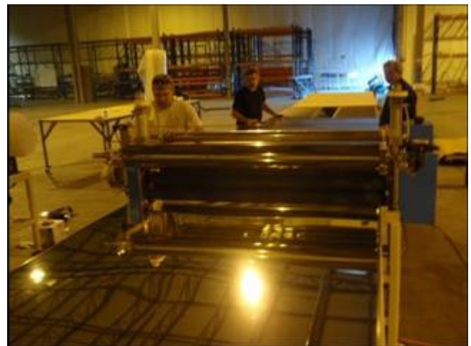
Fig. 3: Lamination of polymer film to aluminum sheet copyright 2010, American Solar Energy Society, all rights reserved
