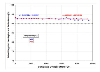
Fig. 8: UAWS exposure of RT-4 samples at 30 and 60°C. Neither SWHR data set dropped below 90%.
