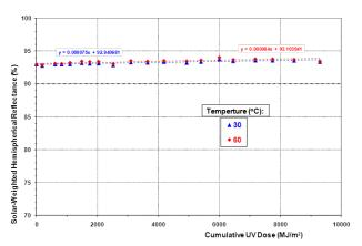
Fig. 10: UAWS exposure of RT-5 samples at 30 and 60°C. The SWHR of neither data set has dropped below 90%.
