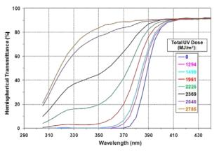
Fig. 2: Spectral transmittance of prototype UV screening film as a function of total UV dose (Ci5000).
