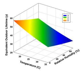
Fig. 11. Outdoor lifetime vs. temperature and relative humidity, based on 300 MJ/m2/y UV irradiance.
