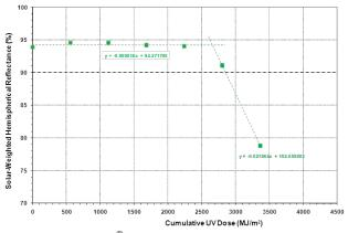
Fig. 4: ACUVEX<sup>®</sup> exposure of RT-2 samples under time varying environmental conditions.
